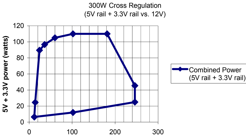
Figure 6 Cross Loading Graph for 300W Configuration Efficiency General
