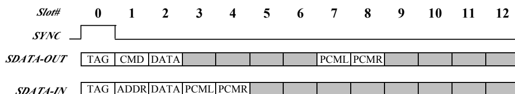
Fig5.2-2 ALC100 slot arrangement – CODEC ID = 10
